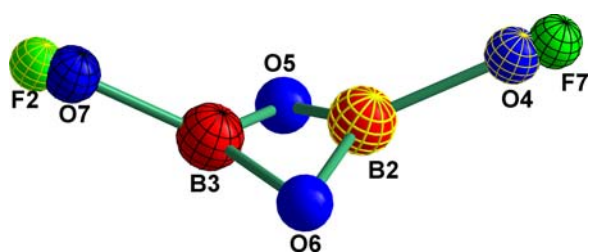
Fig. 2 (color online). Disordered [BO_3]^{3-} group. In the crystal structure of RE_2(BO_3)F_3 ( RE = Tb, Dy, Ho ) the [B(2)O_3(5,6,4)]^{3-} and the atom F2 is represented by an occupation of 65% for Dy_2(BO_3)F_3 and by 67% for Tb_2(BO_3)F_3 and Ho_2(BO_3)F_3 .
