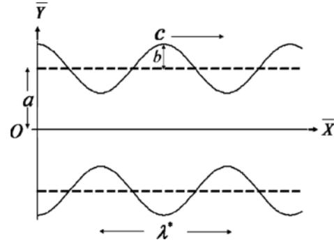
Fig. 1. Schematic diagram of the flow geometry for  $a = 1$ ,  $b = 0.4$ ,  $\lambda^* = 2$ , and  $t = 0$ .
