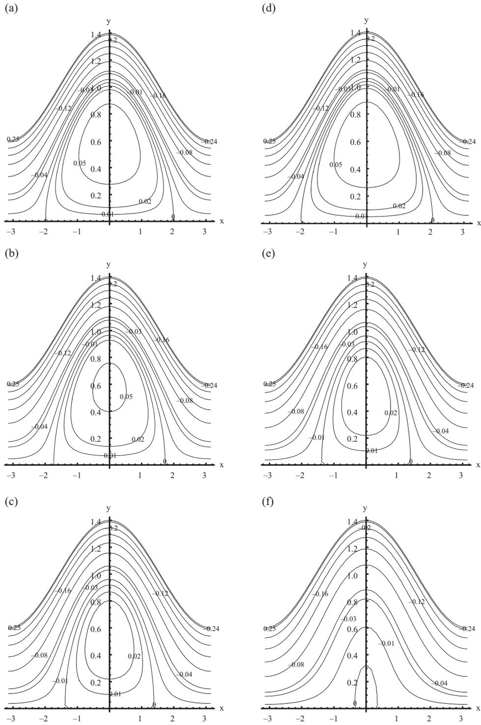
Fig. 5. Streamlines for different values of  $\alpha$  ( $= 0.05, 0.2, 0.5$ ), (left)  $We = 1$  and (right)  $We (= 0.3, 1, 2)$ ,  $\alpha = 0.5$ . The other parameters are  $F = -0.25$  and  $\phi = 0.4$ .
