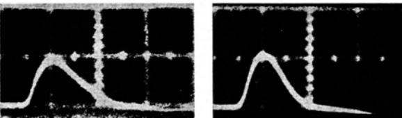
Fig. 2. Several superimposed pulses of a) oscillator (vertical: 2.5 kW/div.; horizontal: 5 ns/div.); b) amplified output (vertical: 45 kW/div.; horizontal: 5 ns/div.).
